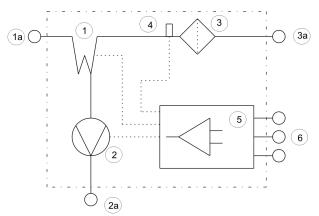
The gas to be conditioned is fed directly into the inlet of the stainless steel, glass or PVDF heat exchanger (1, 1a). A hose is pre-installed between the heat exchanger outlet and the fine filter (3). Sample gas is continued directly from the outlet of this filter via hose fitting (3a).
