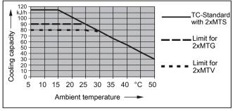
Remark: The limit curves for the heat exchangers exchanger PTG, PTV or MTV apply to a dew point of 40  $^{\circ}$ C.
